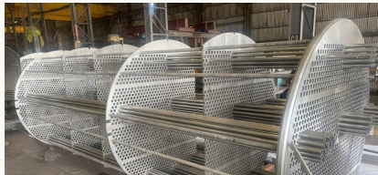
Tube bundles ready for shell Stainless tube nests with baffles and tie rods
