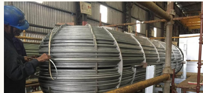
U-tube bundle assembly Bundle strapped and checked before insertion
