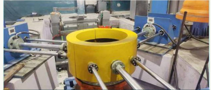
Clamping cylinders along with power packs are used to hold the autoclave in position
