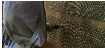
Tube-to-tubesheet expansion Rolling and leak testing in the shop
